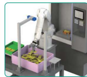
Picking from a large pallet (Fixed camera)
